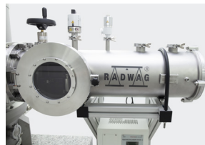
LOAD LOCK - Switching and adding artefacts without opening of the main chamber
