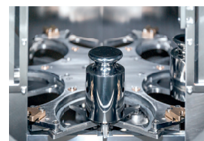
Suspended weighing pan of custom design eliminating eccentricity errors
