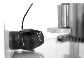
Additional circulator eliminating air bubbles
