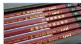
Testing Pencil Apply to DIN or JIS spec. 17-grades hardness (6B-6H)
